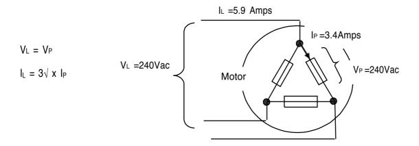
Therefore, the Line current or Full Load Current of the motor when connected in 240V Delta is <u>5.9Amps</u>. A Variable Speed Drive capable of a continuous output of 5.9 Amps is required.
