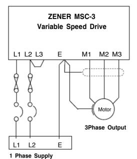
Speed control can be manually using the controls provided or remote speed potentiometer. A Pressure control system can be easily achieved using the drives internal PID control and an external pressure transducer.
