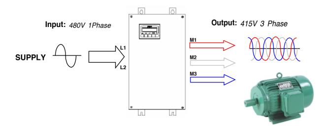
**1. 240V 1Phase Supply:** The ZENER VSD (or equivalent) takes the 240V single phase AC Supply and converts it to a 3 Phase output suitable for a standard 3 phase 240V motor.
